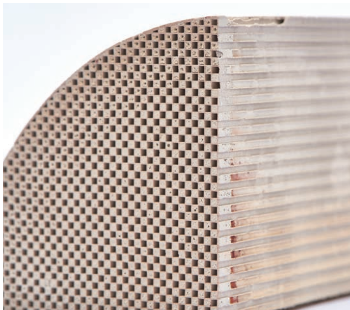
Left: Gasoline particulate filters rarely need active regeneration as soot is continuously burned off in the exhaust system
